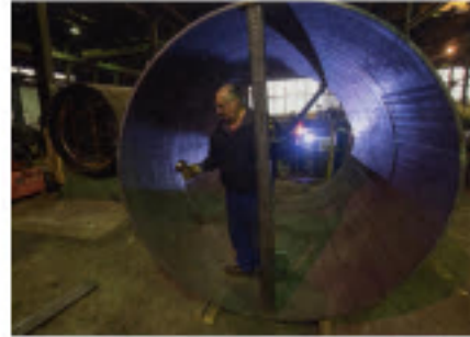
Contractor Gary Bensman inspects a boiler course for a new Pennsylvania Railroad T1 duplex. Steve Smedley
